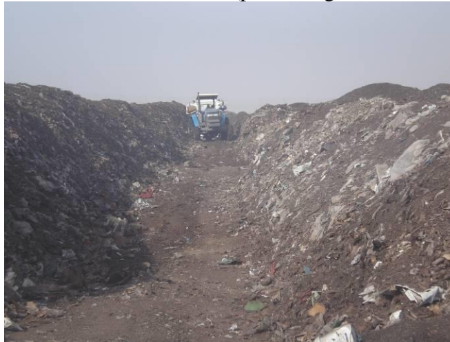
Contaminants in windrows (plastic bags, buckets, etc.)
