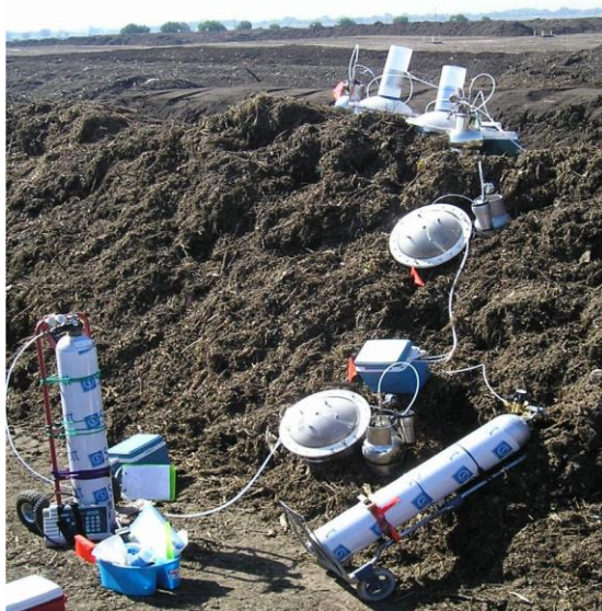
U.S. EPA Surface Isolation Flux Chamber Assembly
