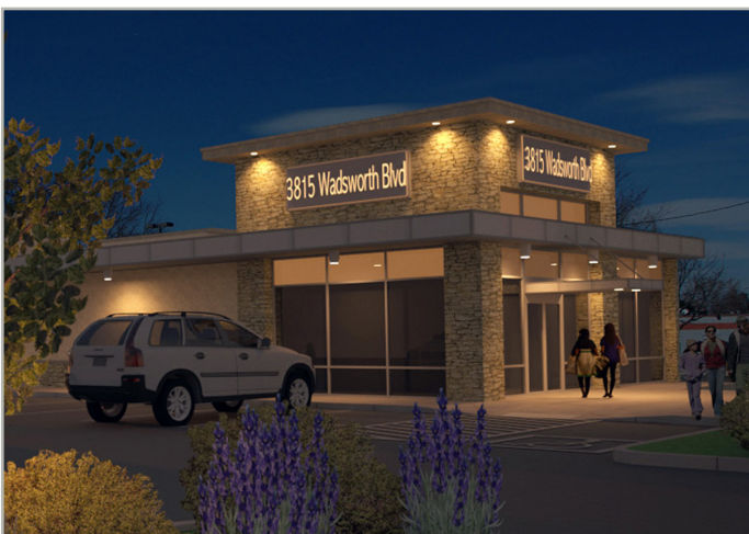
Example of lighting aimed solely at the sign to be illuminated.
