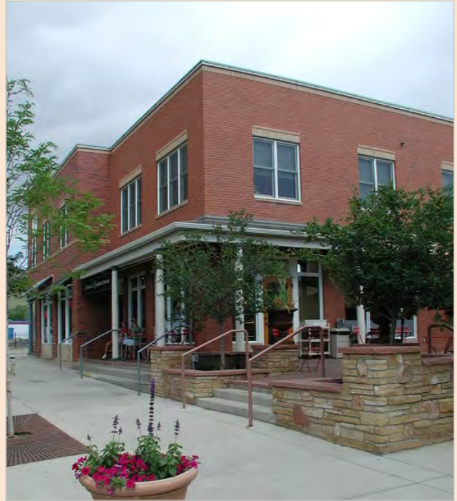
A mixed-use "Main Street" commercial building showing variations in simple massing. Larger windows are used for ground-level retail, while smaller windows are used for second level offices or residences.
